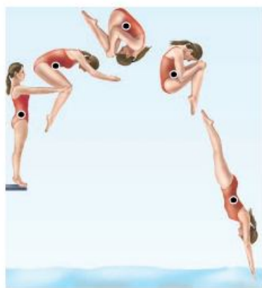
FIGURE 8-29 A diver rotates faster when arms and legs are tucked in than when they are outstretched. Angular momentum is conserved.
