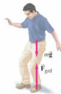
FIGURE 7–12 Example 7–6. When the person lands on the ground, the average net force during impact is \bar{F} = F_{\text{grd}} - mg , where F_{\text{grd}} is the force the ground exerts upward on the person.
