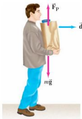
FIGURE 6–2 The person does no work on the bag of groceries since \vec{F}_P is perpendicular to the displacement \vec{d} .
