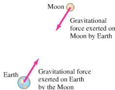
FIGURE 5-19 The gravitational force one object exerts on a second object is directed toward the first object, and (by Newton's third law) is equal and opposite to the force exerted by the second object on the first.
