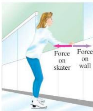
FIGURE 4–9 An example of Newton’s third law: when an ice skater pushes against the wall, the wall pushes back and this force causes her to accelerate away.
