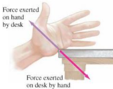
FIGURE 4–8 If your hand pushes against the edge of a desk (the force vector is shown in red), the desk pushes back against your hand (this force vector is shown in a different color, violet, to remind us that this force acts on a different object).
