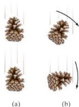
FIGURE 2-1 The pinecone in (a) undergoes pure translation as it falls, whereas in (b) it is rotating as well as translating.
