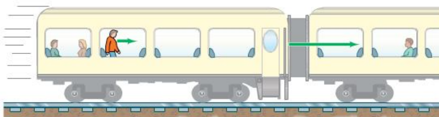
FIGURE 2-2 A person walks toward the front of a train at 5 km/h. The train is moving 80 km/h with respect to the ground, so the walking person's speed, relative to the ground, is 85 km/h.
