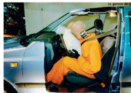
FIGURE 2–14 An air bag deploying on impact. Example 2–8.
